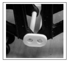
12 The load spacer may is used to space the girders and give the car a level appearance. (Unpainted parts shown for clarity.)
