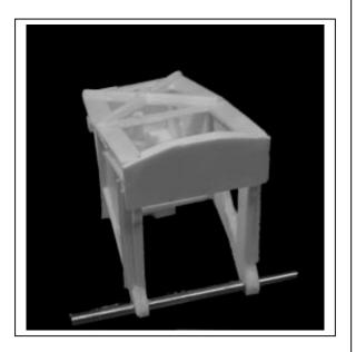
11 The empty car links may be used to run the car empty as shown. (Unpainted parts shown for clarity.)
