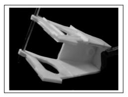
**6** If you are making the car like the photos, trim away the top part of the girder to attach as shown in the adjacent photo. If you wish to make the car per print, Cut back the top brace assembly. In any event the brace should be installed flush with the girder box end and the sides should hang over equally.
