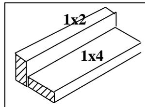
A gluing fixture is a great aid to assembly. It helps hold parts square while gluing.
