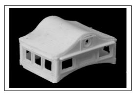
11 Cut and add the roof walk with the cupola just setting on the roof. Cut the roof walk strip to leave a small overhang at the ends. I glued it directly to the roof since my own rolling stock gets handled at a club. You can prop up the roof walk with .030" square styrene to give a more accurate appearance. Add the End Walk Roof Platforms (16) as shown. Don't install ladders until painting and glazing is complete.
