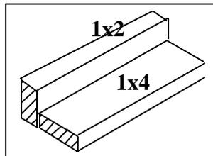
A gluing fixture is a great aid to assembly and marking the longitudinal lines on the tank body. It helps hold parts square while gluing.
