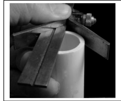
**2** Use the provided template to mark the location of the reinforcing rings on the tank tube. Measure the location of the stub sill 6 scale feet and mark as shown.
