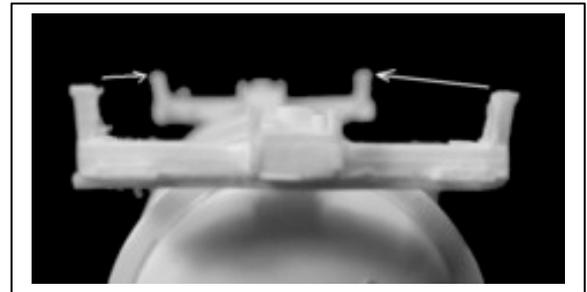
5 Install the Tank Saddle Braces (12) at the bolster/truck location point as shown.
