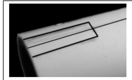
**3** Cement the Tank Pressure Ends (3) to the tank tube. One end will have markings for installing the brake mechanism mount. Orient as shown. Label this as the "B" end.
