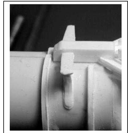
6 Drill a #76 hole at the tip of the Tank Saddle Braces and thread .020" music wire through the holes. Cement in position at the ends. The pictures at the front of this document show three braces per side. Use Athearn Stanchions for a durable support that will withstand club handling.
