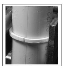
3 Install the Hi Pressure Ends (1). The one with the indentations belongs on the B-End of the tank tube.
