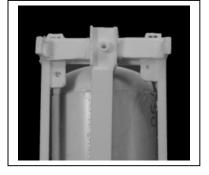
5 Cement the end sills to the tank as shown. The trailing edge of the deck should be in a line with the car end. The ends should line up parallel as shown. Remove the trailing segments of the end sill. They are not used on this car. (Even though shown in some of the common photos throughout.
