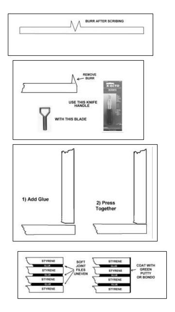
5 Styrene laminations may be built up to make a shaped pattern. In these case Bondo is preferred since it "machines" well and easy to carve with a moto-tool and finish by sanding.
