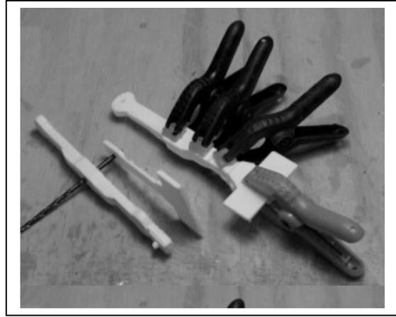
**2** Cut off 1/2 of the tank mounting flange and glue the air tanks (10) to each side of the truck bolster. The lip in the tank should be even with the seam on the bolster.
