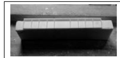
**4** Cement the car ends to the floor sub assembly. Make sure that the tops of the ends are parallel to the floor and that both ends have the same elevation.
