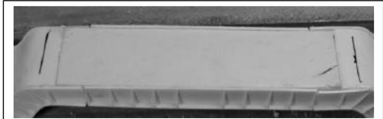
**6** Use a motor tool to create two recesses for adding screws.
