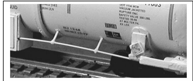
**13** Install the brake valve and brake reservoir as shown. The brake cylinder is attached to the bottom of the tank inline with the brake mechanism behind the truck towards the center of the car. The brake cylinder is cemented on the bottom on the same side of the brake valve. Make sure it will clear the trucks when they are installed.
