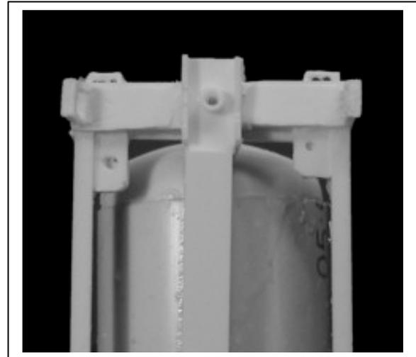
**7** Attach the other end sill making sure that the ends are in parallel alignment.
