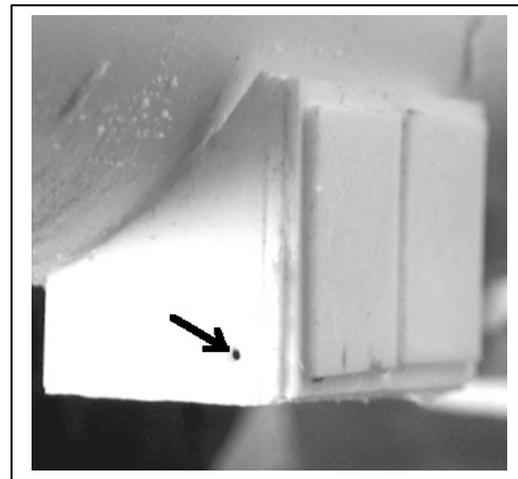
**10** Cement the Control Box Face (8) to the front of the Control Box (7). Fit the control box to the tank. Use of motor tool to trim the supports so that the bottom will be parallel to the track and the face will be close to inline with the tank side as shown on the tank template. Do each side..
