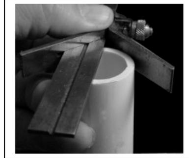
**2** Draw a line the length of the tube. Draw another line 180 degrees from the first. Label one line "top" and the other "bottom".
