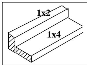
This fixture is a great aid to assembly. It helps hold parts square while gluing and aids in drawing horizontal lines on tanks for tank cars.
