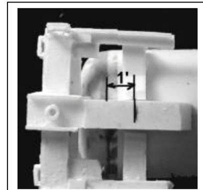
**8** Drill the end of the tank that has the small indentations for pilot holes. Install the brake mechanism mount and Ajax brake mechanism as shown. Install the brake wheel with a small pin. Install the rest of the brake components per diagram.
