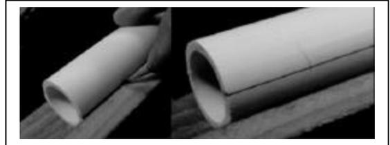
**3** Cement the High Pressure Ends (1) to the tank tube. The "B" end has small indentations for pilot holes. The pressure end piece should be located as shown in step eight where the brake mechanism will be installed. Use Squadron's Green Putty to smooth the joints.
