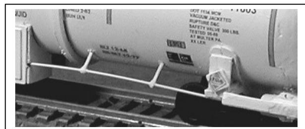
**12** Make a guard railing from .020" steel (not provided) and install as shown in the End Sill (5). It will be necessary to drill with a .020" drill (#76).
