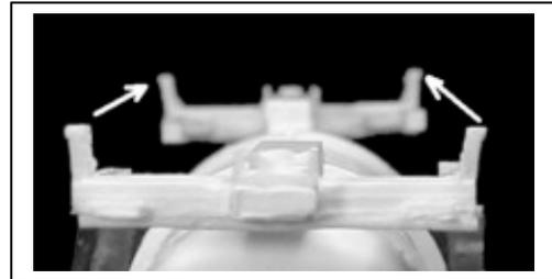
**7** Cut the saddle halves in half. Trim the saddle halves so that the ends. Measure 1' (s.f.) on the tank tube (not the pressure end) and mark for the saddles and the Cut back the side stringers to match the saddle halves when installed at the truck location The saddle halves connect to the bottom of the tank and center sill. The side stringers should be cemented to the saddles.
