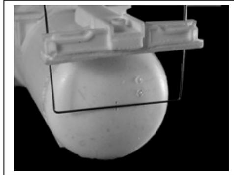
**13** Install the brake valve and brake reservoir as shown. The brake cylinder is attached to the bottom of the tank inline with the brake mechanism behind the truck towards the center of the car. The brake cylinder is cemented on the bottom on the same side of the brake valve. Make sure it will clear the trucks when they are installed.
