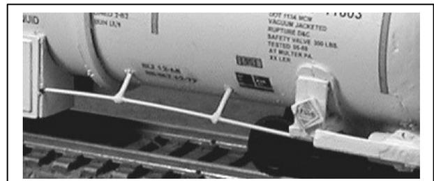
**11** Cement the Control Box Face (8) to the front of the Control Box (7). Fit the control box to the tank. Use of motor tool to trim the supports so that the bottom will be parallel to the track and the face will be close to inline with the tank side as shown on the tank template. Do each side..
