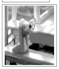
18 File the boss on the Air Tank until it is flat; then attach to the inboard end of the Main Span Bolster as shown. Add the smaller air tank opposite the main air tank. (Not shown)
