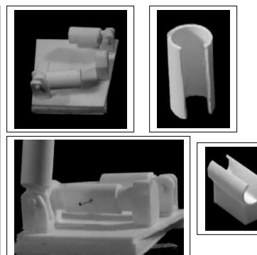
14 Install the Hyd. Pistons (15) on the main girder assembly – 4 places as shown on the one end photo.
