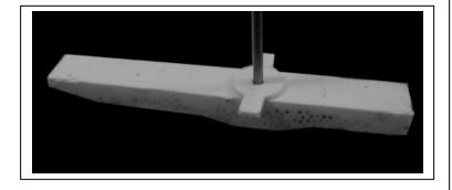
2 Attach the Bolster Flanges (21) to the Main Span Bolster as shown. The center one points up and tucks under the Bearing Mount extention. Trim to match the Bearing Mount. Two more are placed to engage the truck bolsters as shown.
