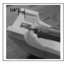
3 Match the Girder Core to the assembled ends and drill as shown in the next step. The core should be filed as necessary to get a good fit. Do not cement yet.
