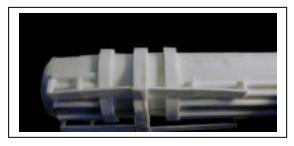
6 Clip the part of the template as shown and apply to the tank tube. Rubber cement is a good solution since it can be removed with lighter fluid. Use the side view on the template to locate the upright stanchions. Start with a #72 drill and enlarge as necessary for the upright stanchions.
