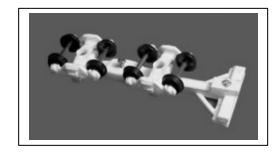
10 Glue the brake mechanism to the brake stand as shown. Install the brake wheel using the small pin. Cut the pin off and use an emery wheel on a motor tool to smooth it.
