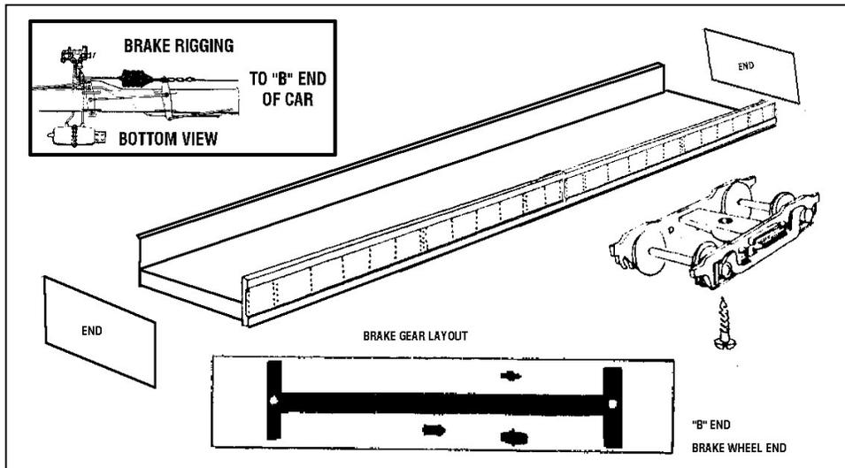
**3** Attach coupler mount to completed car. It may be necessary to file the ends to get a fit. Use the 1/8" screws to hold the coupler cover. Work carefully as the threads are delicate. Do not apply couplers until the model is painted.
