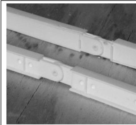
7 Using temporary 1/8" brass rods, Thread on the inside brace supports and the tension beams as shown. Remove the bosses at the ends of the tension beams and cement the inside brace supports to the tension beams
