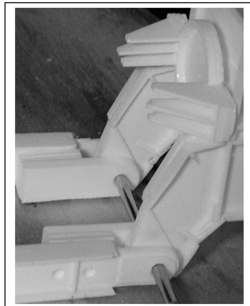
5 Insert the plugged end of the compression spacer assembly and insert into the end of the tank assembly. Prepare the remaining end as previous and install using ACC cement.
