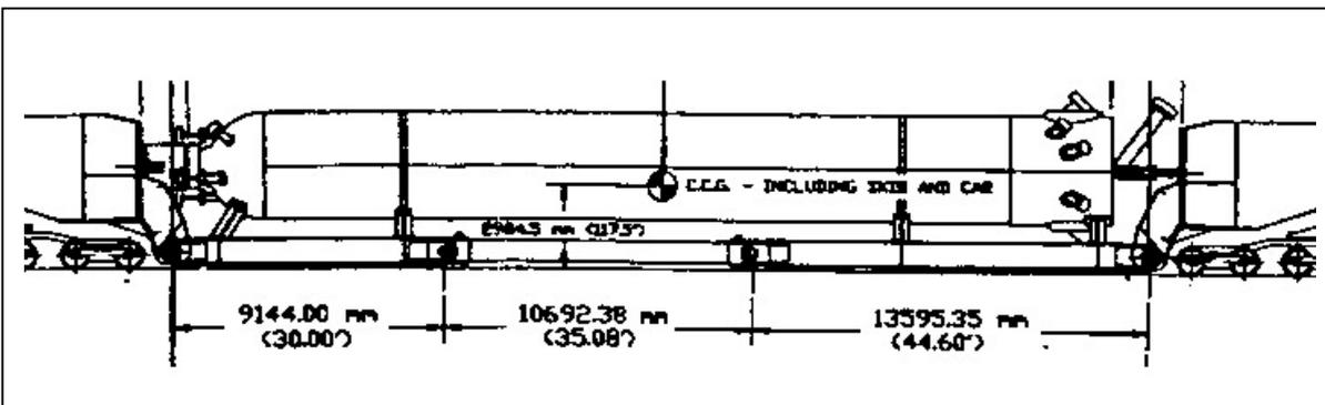
**7** Determine that the load is being held straight and level by the compression braces and spacers.
