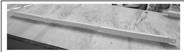
4 Using temporary 1/8" brass rods, Thread on the inside brace supports and the tension beams as shown. Remove the bosses at the ends of the tension beams and cement the inside brace supports to the tension beams
