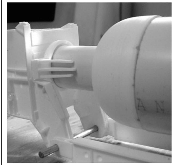
**8** Install the small brace at the end and the large braces in the center as shown. The braces are positioned against cast-on bosses on the inside of the tension beams and set the width. Replace the brass fitting rods with the two short styrene tubes at each end. It is suggested that the tank be cemented to the braces for maximum stability.
