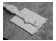
Add the brake wheel to the brake stand with the small pin provided. Attach the end fascia and then cement the a brake stand assembly to each car end as shown. Add the brake valve, break reservoir and auxiliary air tank as shown to the B end of the car. If you wish to add piping, the adjacent photo is the only information we have. My choice is always .015 steel since it resists bending once the model is finished and placed in operation.
