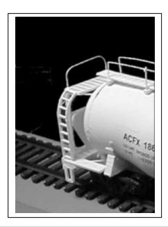
14 Add the Shield to the inside of the End Frames by cementing to the End Frame and the Deck. Add brake details as shown. Ad the Placard Mount to the side of the car at about 1/3 of the distance from the end and just below the tank centerline. After painting, add couplers of your choice.
