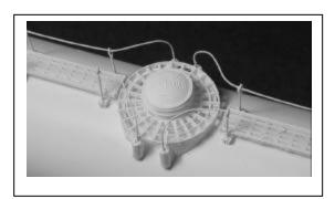
13 Add the ladders. Bend by applying heat. (Microwave in increments of 10 seconds or swipe your wife's curling iron.) Prototype photos shown one sharp bend just about the center of the ladder rather than the curved technique I used. My mistake.
