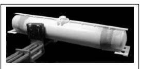
10 Add the End Frames by cementing to the end deck. Add the Brake Mechanism Mount to the B End of the car.
