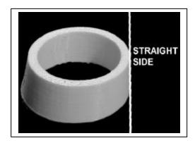
3 Apply the short section of tubing and smooth the transition with Squadron's Green Putty.
