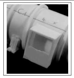
9 The stub sill should be cut to 9 scale feet (away from the coupler pocket) if it hasn't been done already. This is a stock casting.
